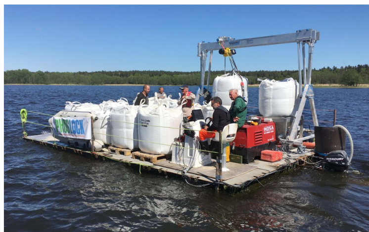
Figure 6. Treatment to a large waterbody using a crane fitted pontoon system.
