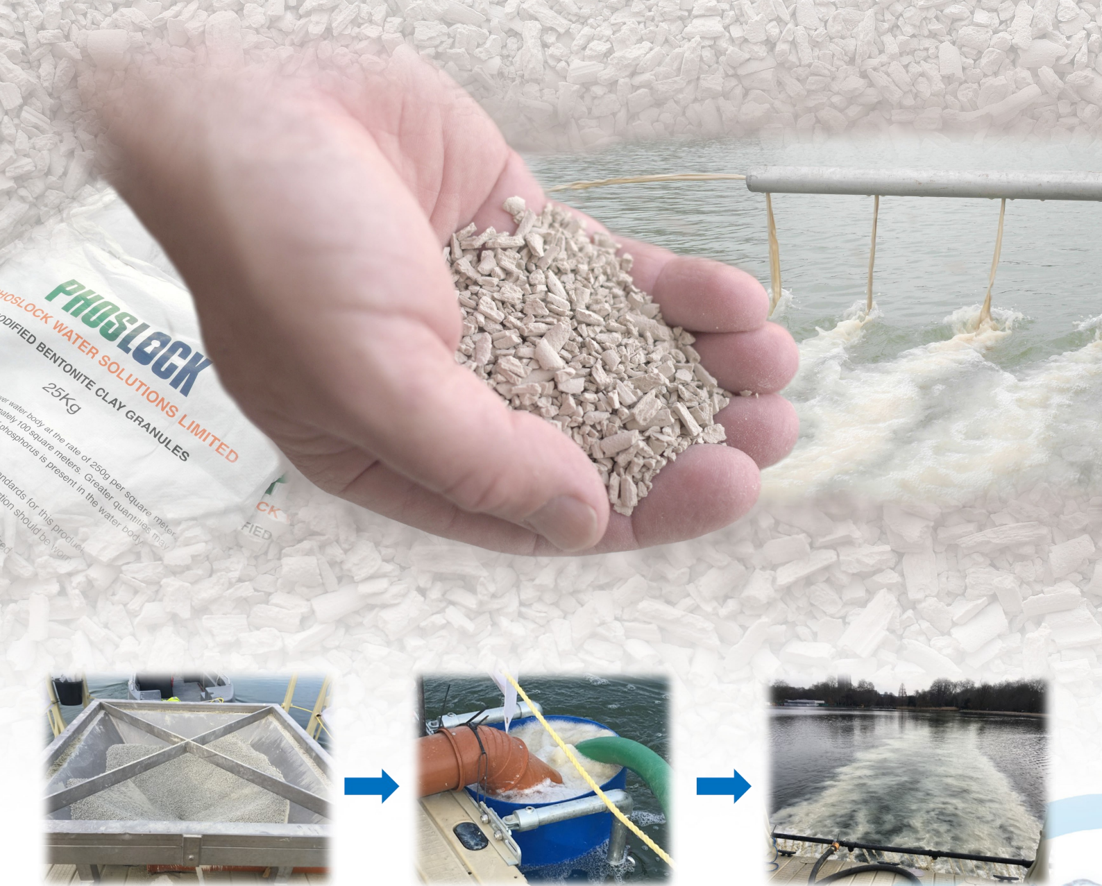
Figure 4. Diagram of the Phoslock application process, with Phoslock in its granule form (left), granules being mixed with lake water (middle) and then applied to the surface of a waterbody (right).
